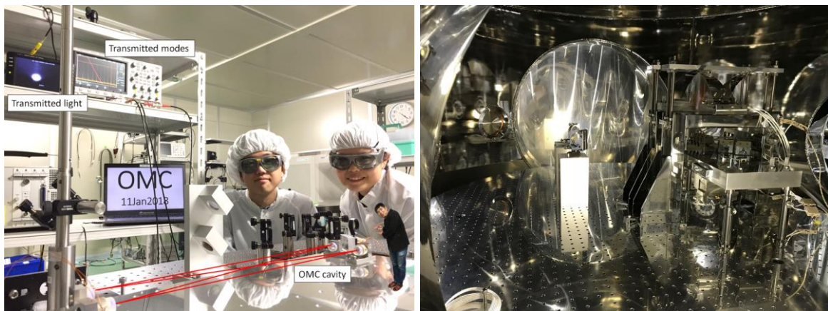
Fig.1 Left: assembly of the OMC at Tokyo Tech, Right: Installed OMC in the vacuum chamber.
