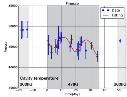
FIGURE 1. Measured finesse oscillations. Depending on the thickness of the adlayer on the cooled mirror, the finesse of the optical cavity which was put inside the KAGRA cryostat changed.
