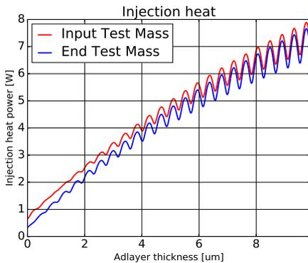
FIGURE 2. The estimated heat injection to the test masses in KAGRA. An adlayer absorbs a part of circulating laser, and it causes the additional heat to the test masses.
