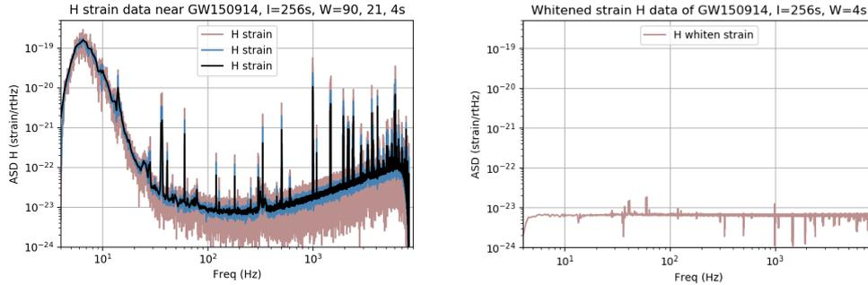
Figure 1: ASD of raw data from Hanford on the left, in the range from 4 to 9000Hz, for the interval of 256s around the time of the event with 90s windows. where one can observe the cutoff at the Nyquist frequency. On the right, the strain after applying the whitening filter, as explained in the public LIGO python scripts.
